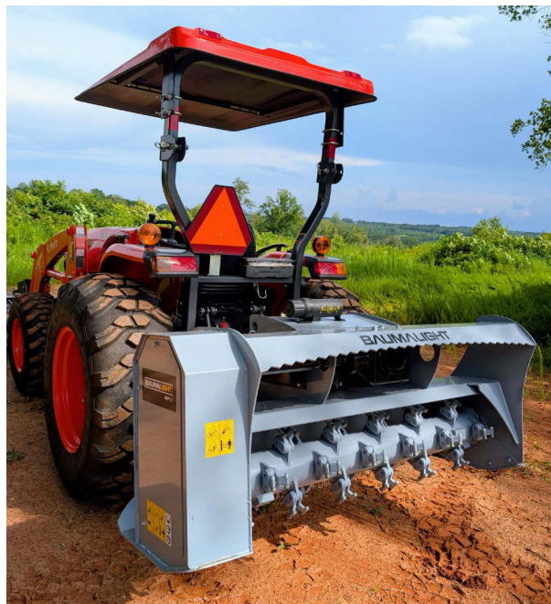
Owner-operated tractor and forestry mulcher used for access, brush management, field preparation, and land stewardship.
